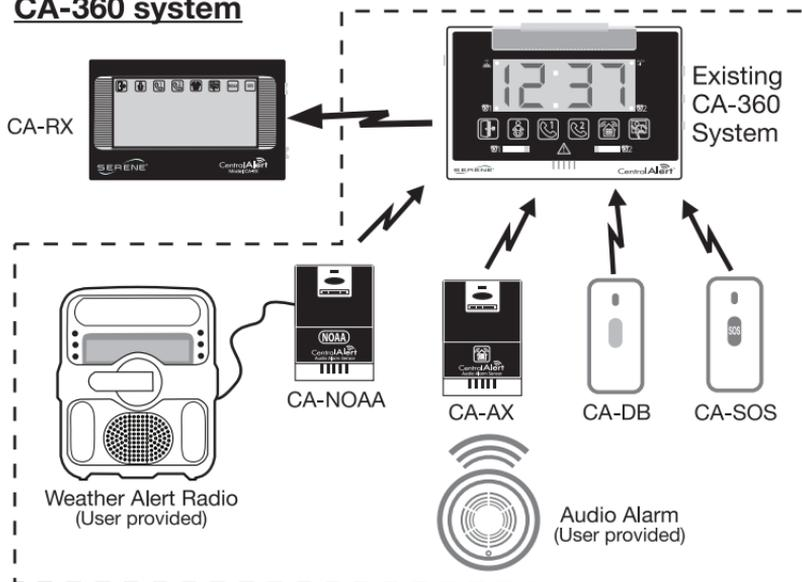
This is a typical application for adding a CA-RX remote receiver to a CA-360 system in order to improve user convenience and coverage area.
