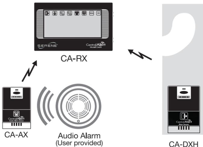
Application 2 demonstrates how a simple wireless notification system can be created using CA-RX. It notifies you when someone is at the door, or if an audio alarm is activated. The entire system is compact, light weight and is ideal for travelling use.
